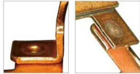
Welding of Copper (Cu) Bus Bar
