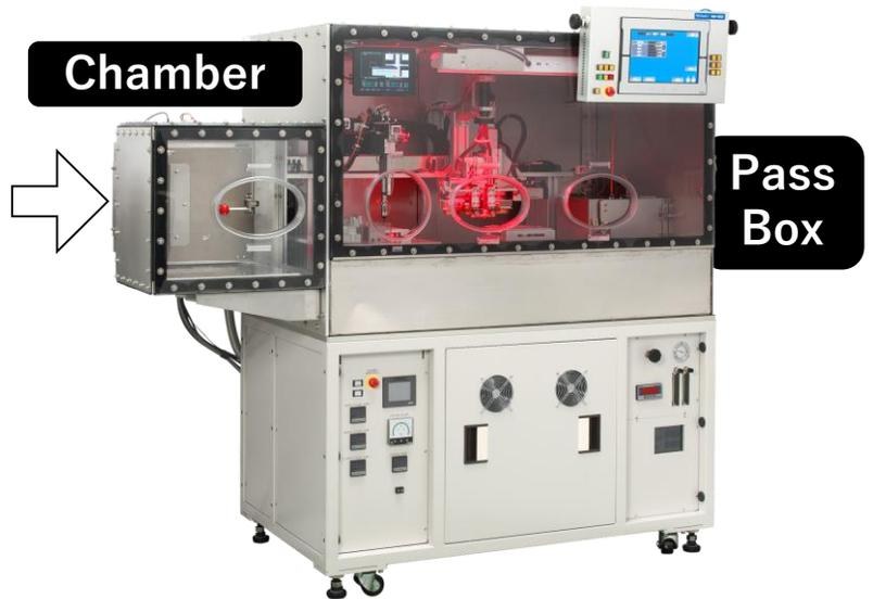
Anneal chamber can be attached to right and/or left side
