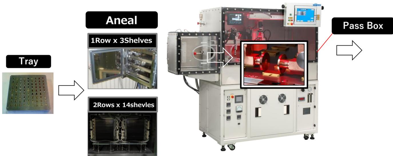
Anneal chamber can be attached to right and/or left side
