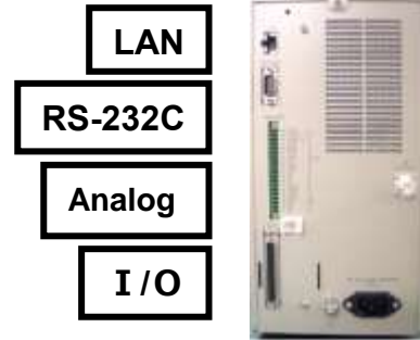
Generator rear face
